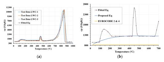
**Figure 10.** Specific heat: (a) comparison of the experimental and proposed specific heat equations; (b) comparison of proposed equations, simplified equation, and Eurocodes 2 and 4 values.
