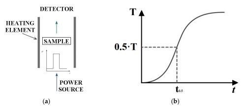
Figure 2. LFA method: (a) configuration of test; (b) calculation of parameters.
