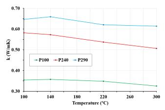
Figure 4. Thermal conductivity for LWC-1 at different pressures (100, 240, and 290 N/cm<sup>2</sup>).
