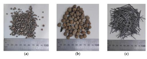
Figure 1. Types of aggregates: (a) expanded clay-fine; (b) expanded clay-coarse; (c) polyolefin fibers.
