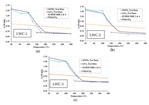
Figure 11. Comparison of the experimental and proposed thermal conductivity: (a) LWC-1; (b) LWC-2; (c) LWC-3.
