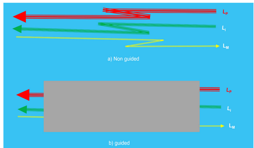
Figure 2. Illustration of the optical channel of a photonic sensor. According to the media used to transmit the Light to and from the object: (a) non guided optical channel and (b) waveguide optical channel (typically optical fiber cables). Courtesy of the author.
