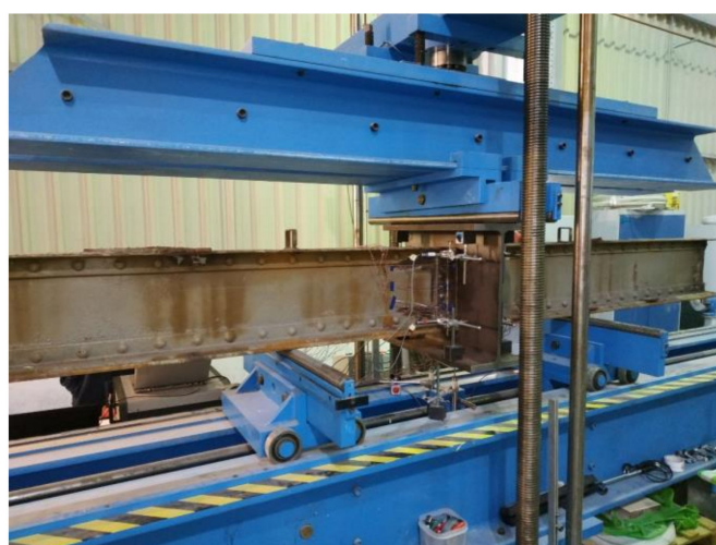
Figure 7. Laboratory test of the non-strengthened connection.
