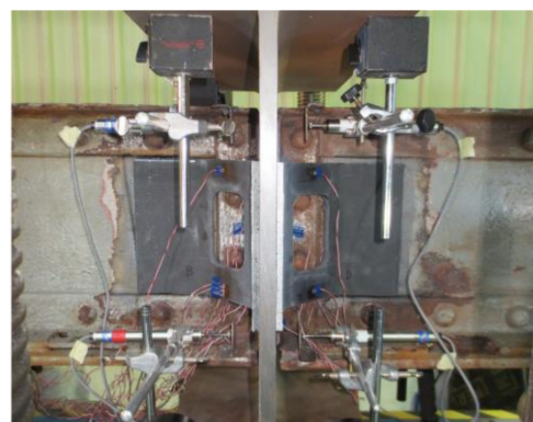
Figure 24. Test of the CFRP-strengthened connection.
