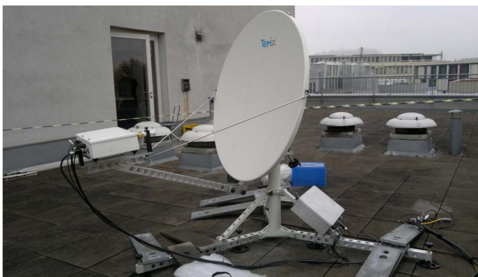
**Figura 2 - Antena Flyaway**
