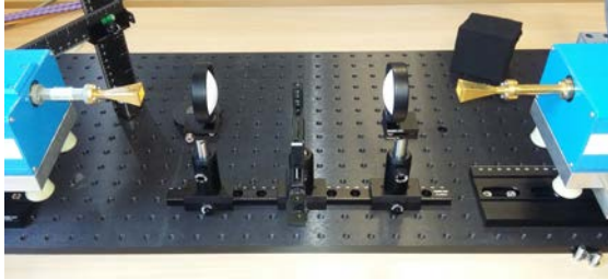
Fig. 16. W-Band quasioptical system with 4f topology ( f = 75 \text{ mm} ). Mm-wave Extension modules V10VNA2 WR-10 (OML), horn antennas and PTFE lenses.
