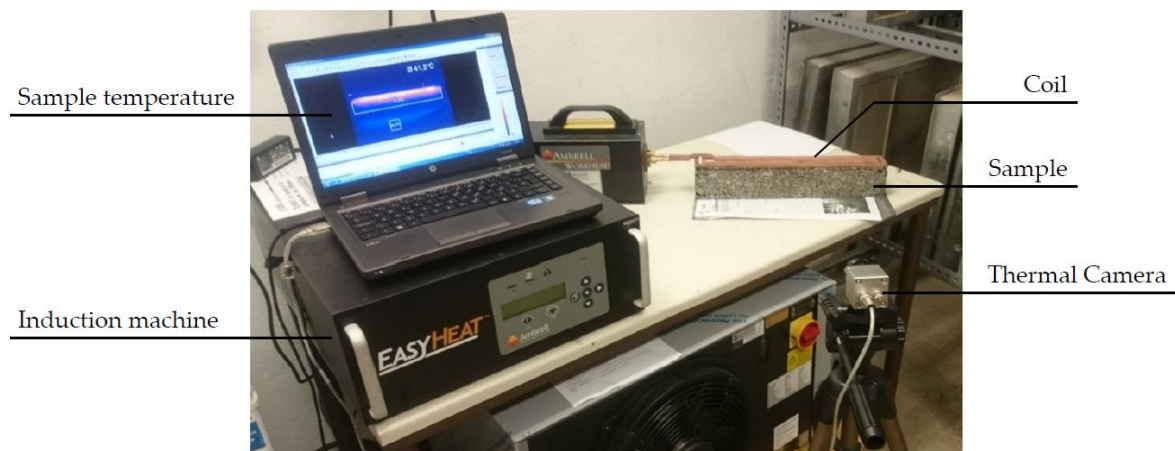
Figure 2. Induction machine with the fatigue test configuration.
