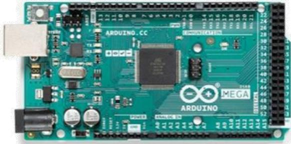
Figura 23: Arduino Mega 2560. [24]
