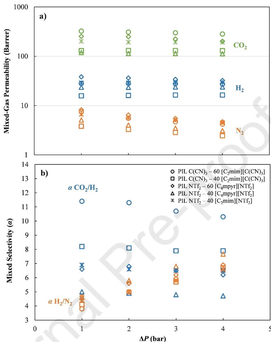
**Figure 7.** Experimental mixed gas a) permeabilities and b) permselectivities as a function of total feed pressure at  $T=35\text{ }^\circ\text{C}$ , through the PIL-IL membranes studied in this work.
