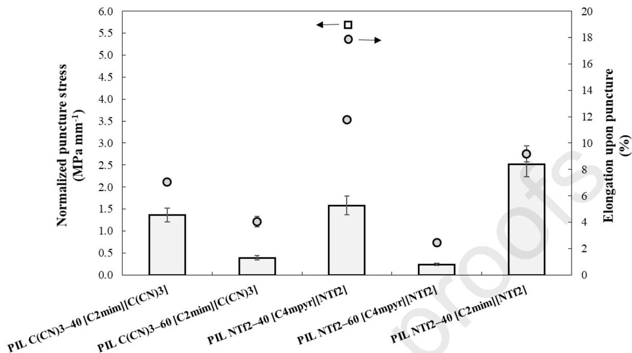
**Figure 2.** Normalized puncture stress ( $\text{mPa mm}^{-1}$ ) and elongation upon puncture (%) of the studied PIL-IL membranes.
