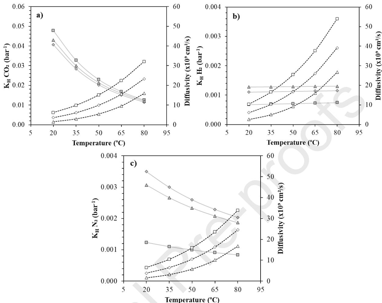
**Figure 5.** Henry's equilibrium constant ( $K_H$ ) (filled symbols) and gas diffusivity coefficient in IL ( $D_i$ ) (white symbols) from COSMO-RS calculations used in Eq. (6). ( $\diamond$ )  $[\text{C}_2\text{mim}][\text{NTf}_2]$ ; ( $\square$ )  $[\text{C}_2\text{mim}][\text{C}(\text{CN})_3]$ ; ( $\triangle$ )  $[\text{C}_4\text{mpyr}][\text{NTf}_2]$ .
