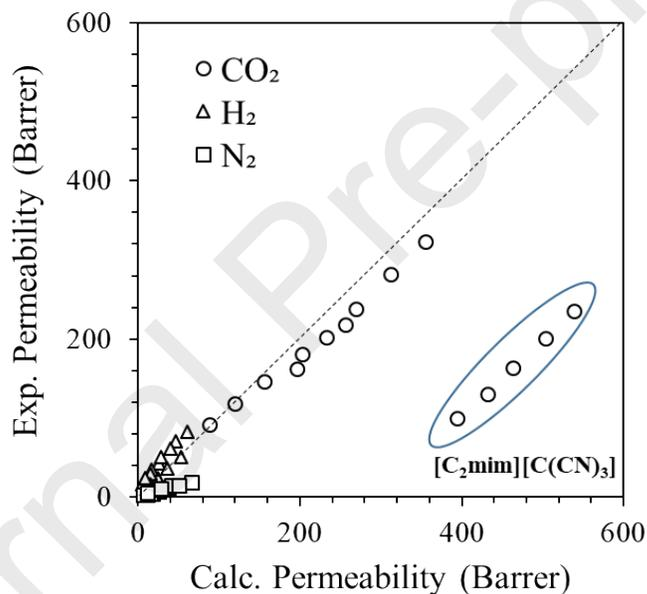
**Figure 4.** Mixed experimental vs calculated (Eq. (6))  $\text{CO}_2$ ,  $\text{H}_2$  and  $\text{N}_2$  permeabilities through PIL-40 IL membranes, at the different studied temperatures and 1 bar of feed pressure.
