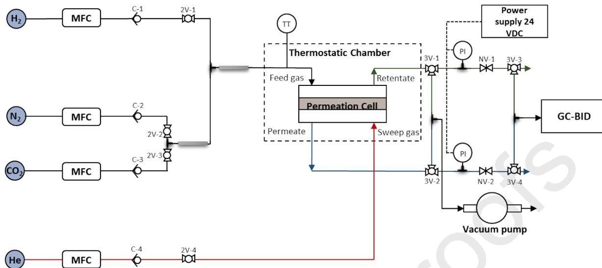
**Figure 1.** Mixed gas permeation set-up. MFC, flow controller; C, check valve; 2V, 2-way valve; 3V, 3-way valve; TT, thermocouple; PI, pressure transducer; NV, Needle valve; GC-BID, gas analyzer. Adapted from ref. [30].
