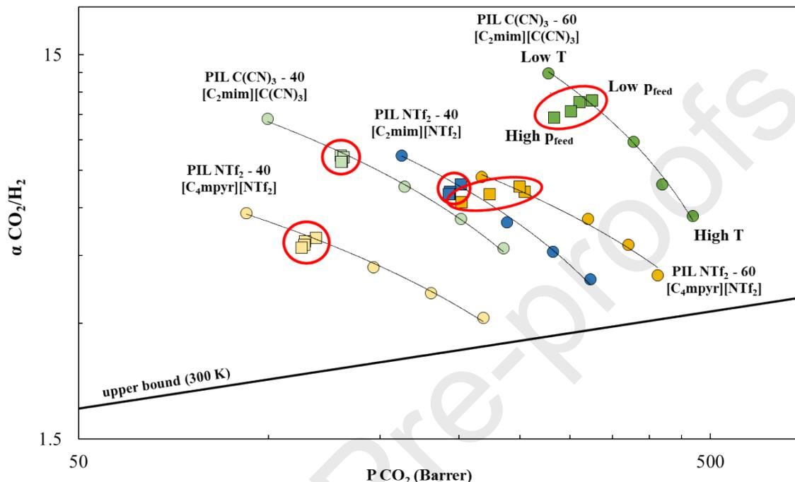
**Figure 8.** Mixed  $\text{CO}_2/\text{H}_2$  separation performance of the PIL–IL membranes studied. The experimental error is within the data points. Data are plotted on a log–log scale and the upper bound at 300 K was adapted from Rowe et al. [45]. Pressure effect on  $\text{CO}_2/\text{H}_2$  separation performance is represented by squares and highlighted with red circles while temperature effect is represented by circles.
