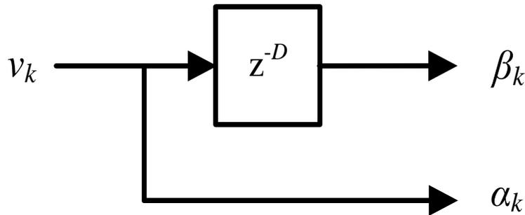
Figure 4. Discrete time representation of the QSG of the transport delay (TD) PLL.
