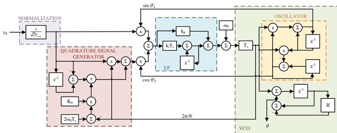
**Figure 16.** Structure of the optimized 2S-PLL [79] used in the Table 5.
