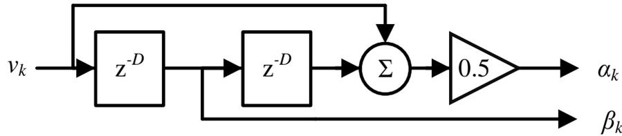
Figure 5. QSG with two delay buffers.
