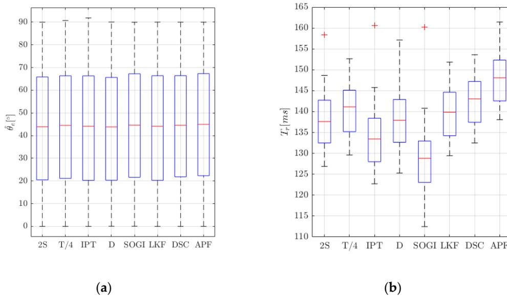
**Figure 14.** Results of MC tests with phase jumps. Starting phase angle and jump magnitude are varied through LHS. (a) Overshoot of the peak phase error and (b) response times.
