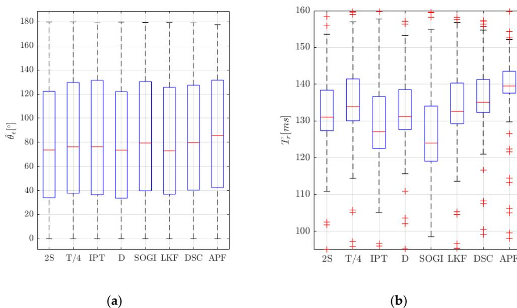
**Figure 13.** Results of MC tests with frequency jumps. Starting phase angle and jump magnitude are varied through LHS. (a) Overshoot of the phase errors and (b) response times.
