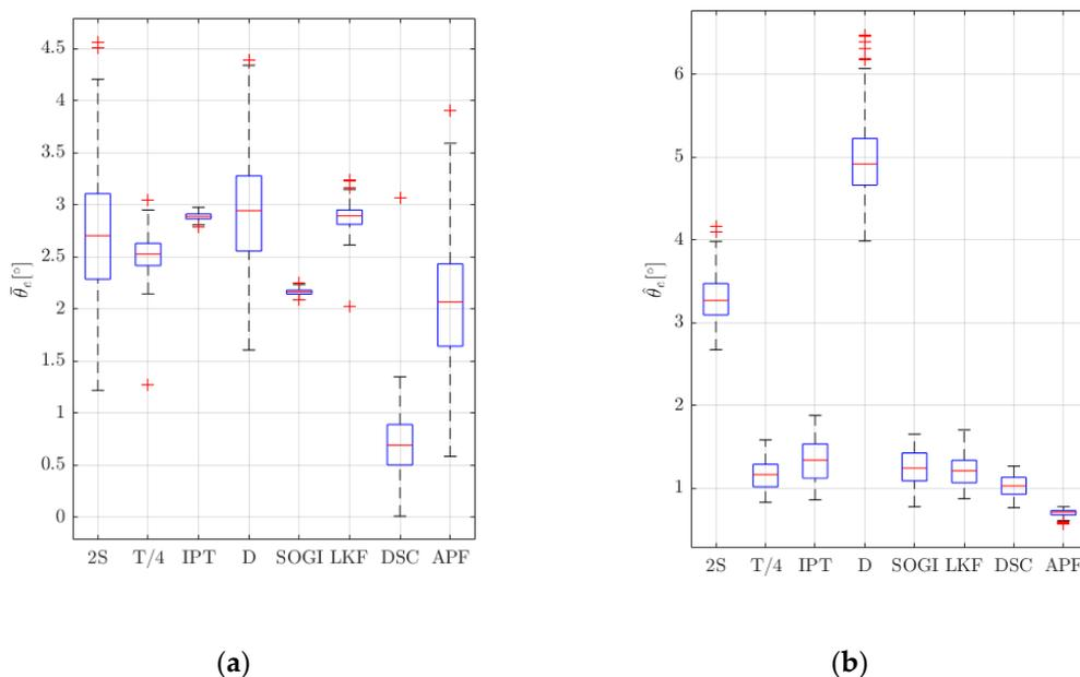
**Figure 12.** Results of MC tests in steady state. Harmonic distortion of the grid voltage and the nominal grid frequency are combined through LHS. (a) Mean phase error and (b) Ripple of the phase error.
