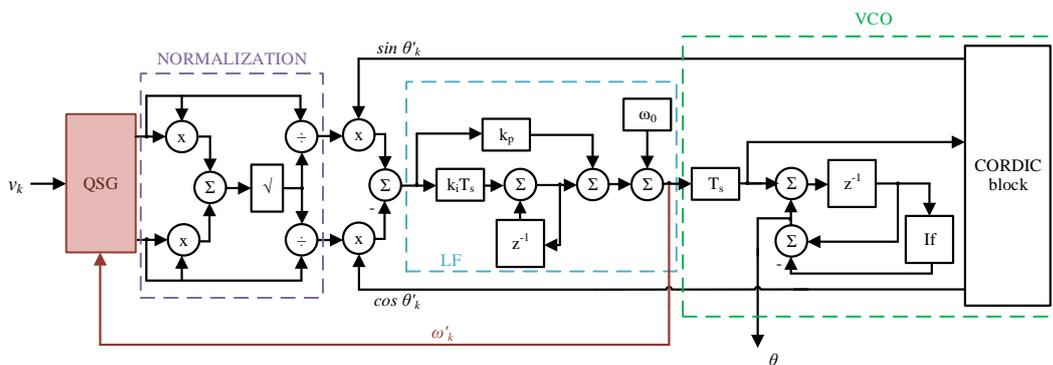
Figure 10. Structure of the PLL used in the tests.
