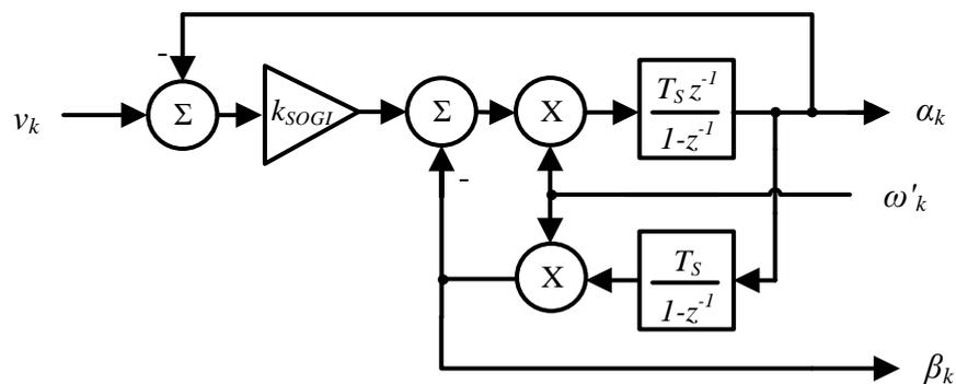
Figure 8. Block diagram of the QSG second-order generalized integrator (SOGI).
