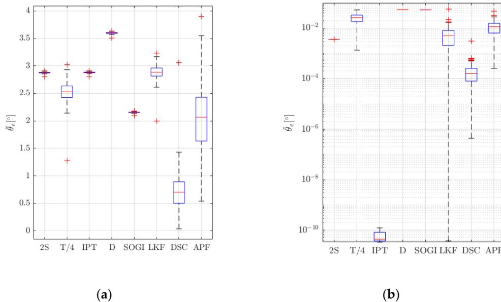
**Figure 11.** Results of Monte Carlo (MC) tests in steady state. Grid voltage and the nominal grid frequency are combined through Latin hypercube sampling (LHS). (a) Mean phase error and (b) Ripple of the phase error.
