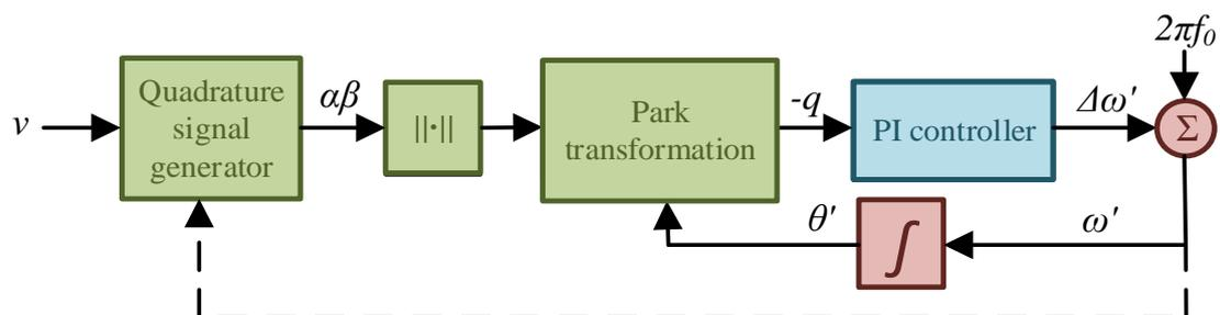
**Figure 3.** General structure of a single-phase synchronous reference frame (SRF) PLL.
