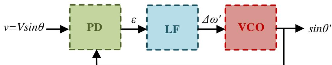
Figure 1. Basic structure of a phase-locked loop (PLL).
