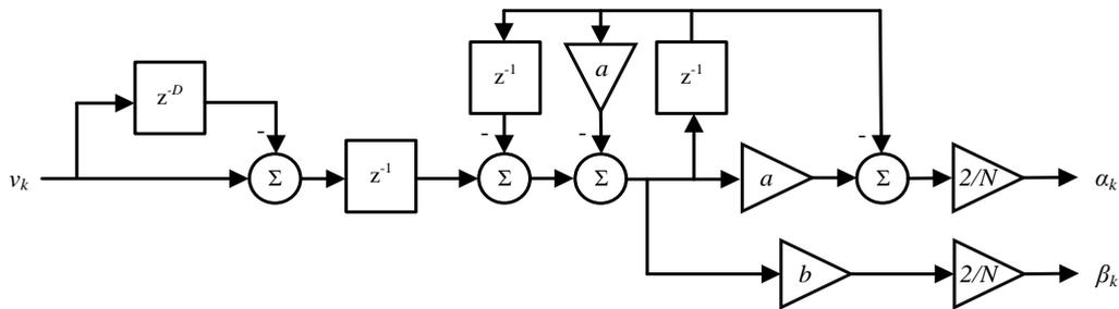
**Figure 7.** Quadrature signal generator with recursive discrete Fourier transform (RDFT) where  $a = \cos(2\pi/N)$  and  $b = \sin(2\pi/N)$ .
