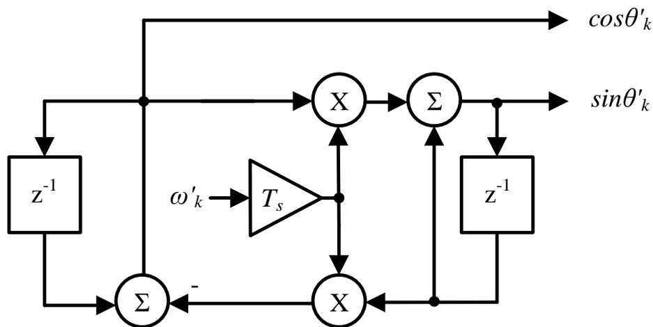
Figure 2. Implementation of the digitally controlled oscillator (DCO) proposed in [27].
