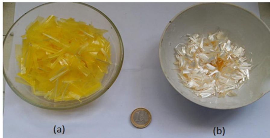
Figure 2. Types of synthetic fibers used in this work: (a) PO/A fibers and (b) PAN fibers
