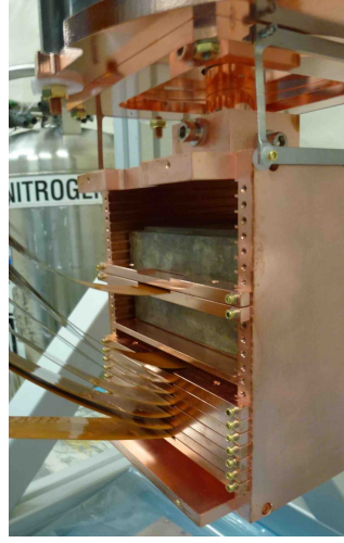
Figure 4.2: Current DAMIC array at SNO-LAB consisting of seven CCDs for a total mass of 40 g. Retrieved from [Set20].
