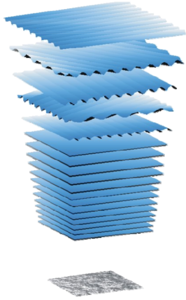
FIGURE A.3: Free surface reconstruction graphically explained as a sum of the different frequencies and directions existent in the analyzed spectrum. Source: (Holthuijsen, 2007).
