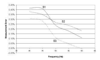
Fig. 5. Measurement error of solid state energy meters under variations in the nominal frequency.
