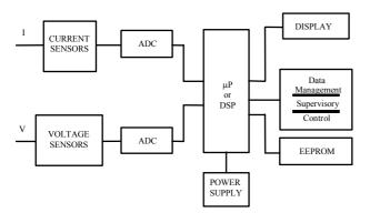
Fig. 1. Basic scheme of a digital sampling based energy meter.
