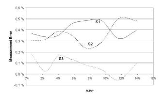
Fig. 4a. Measurement error of solid state energy meters under unbalanced energy.
