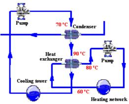
Figure 8.- Cooling circuits and heating systems.
