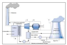
Figure 5.- Schematic diagram of the installation
