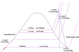
Figure 6.- Steam cycle for the situation where no heating is used.
