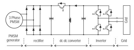
Figure 4. Basic equivalent circuit of the conversion system based on a three-phase PMSM.
