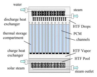
Fig. 2. Diagram of the RHTS concept [9].
