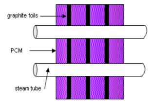
Fig. 5. Scheme of PCM/fins sandwich configuration [11].
