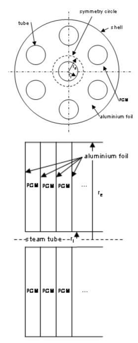
Fig. 4. Schematic of HTLHTES with aluminium foil [8].
