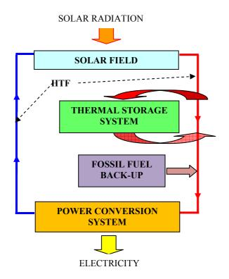
Fig. 1. Diagram of a thermal solar power plant [9].
