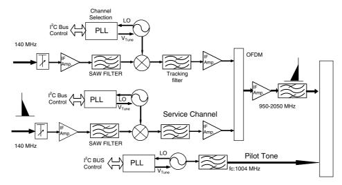
Fig. 7. Up-conventer for the OFDM channels.
