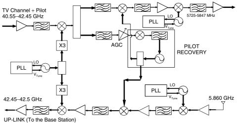
Fig. 11. Block diagram of the local repeater.
