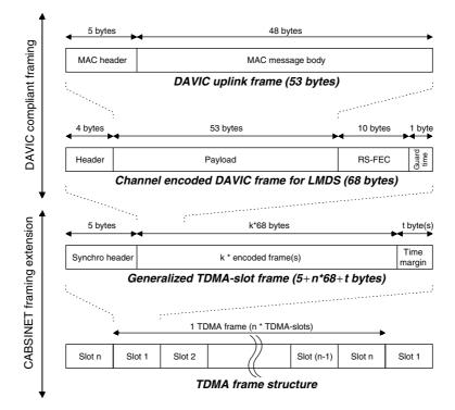
Fig. 4. Extended (eDAVIC) frame structure for more efficient communications and flexibility.
