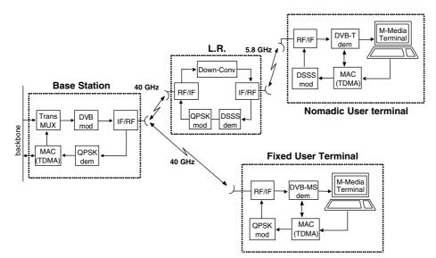
Fig. 2. General structure of CABSINET two-layer entities.
