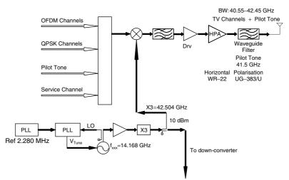
Fig. 8. RF up-converter for the base station.
