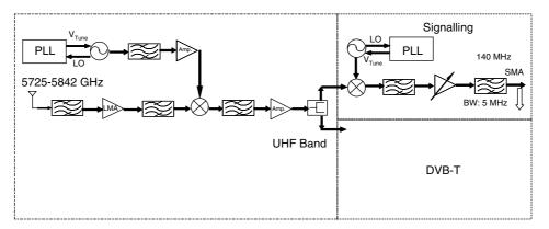
Fig. 10. Block diagram for down-converter of the nomadic terminal.
