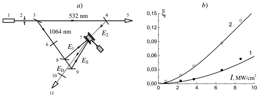
Fig. 3. Experimental setup (a). The diffraction efficiency  $\xi$  versus the intensities of waves involved in hologram recording ( $I_1 = I_S = I$ ) (b) for a thin layer of the dye solution ( $I$ ), and for FPI (2). Circles represent experimental data, lines – theoretical calculation.
