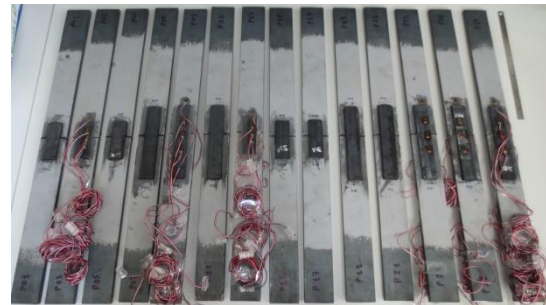
b) Instrumentation with strain gauges
