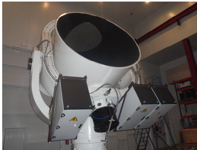
Figure 22. Photo of the MFI mounted on the QUIJOTE telescope.
