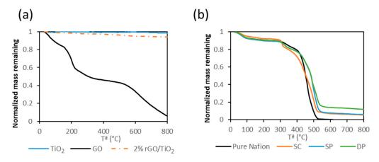
Figure 2. TGA of TiO<sub>2</sub>, pure GO and rGO/TiO<sub>2</sub> (a). TGA of pure Nafion and photocatalytic membranes (b).
