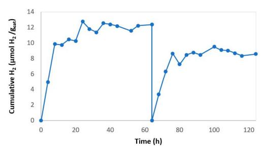
Figure 7. Hydrogen production with reused 2% rGO/TiO<sub>2</sub> SP membrane.
