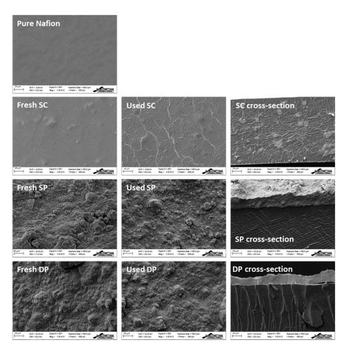
**Figure 4.** SEM images of pure Nafion, fresh membrane and used membrane surfaces, and fresh membrane cross-section. Scale bar =  $10 \mu m$ .
