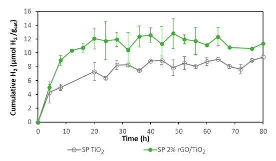
Figure 5. Comparison of hydrogen production with 2% rGO/TiO<sub>2</sub> SP and bare TiO<sub>2</sub> SP membranes.
