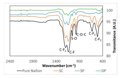
Figure 3. Pure Nafion and photocatalytic membrane FTIR spectra.
