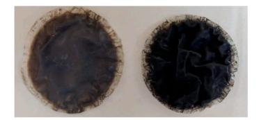
Figure 8. 2% rGO/TiO<sub>2</sub> membrane before (left) and after 96 h of use (right).
