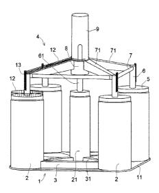
and the center of said lower slab; a metal superstructure supported on the concrete substructure and forming the base for connection with the wind turbine tower, said tower being coupled at the center thereof; and metal covers covering each of the cylinders, on which the metal superstructure is supported and to which vertical pillars are secured, linked together by beams, which join at the central pillar by an element whereon the base of the wind turbine tower is secured.
