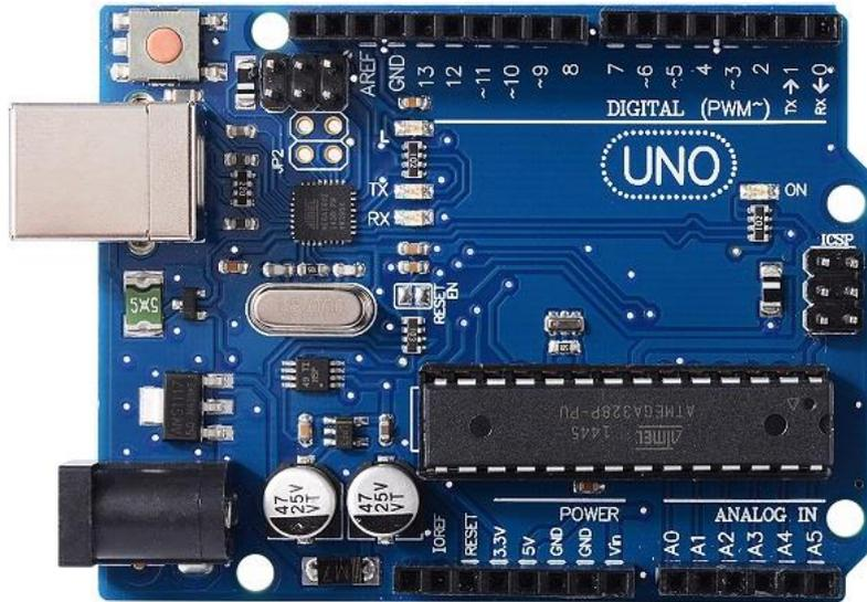
Figura 5-2 Arduino Uno REV3
