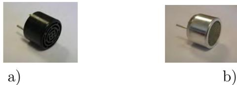
Figura 1.8: a) Sensor Murata 40B8 R/S b) SensComp 40LT16/40LR16
