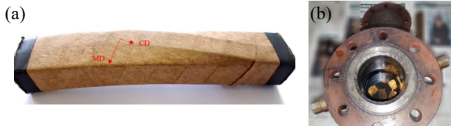
Figure 1. (a) CTC sample with the principal directions of the paper, MD and CD; (b) test pieces in the vessel filled with dielectric oil.
