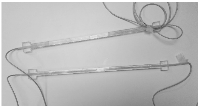
Figure 3 FBG Sensor packaging used in the structure
