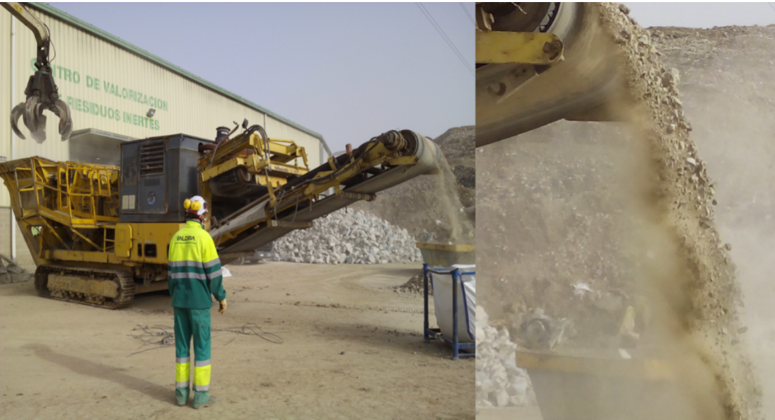
Figure 2. Process of crushing ballast and sleeper waste.
