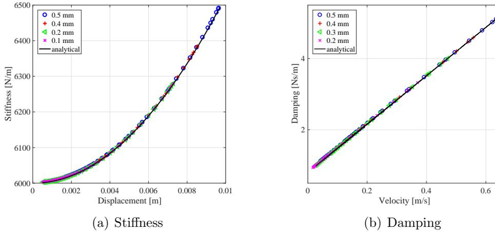
Figure 5. Comparison between the estimated stiffness and damping functions and the analytical equivalent functions: System with combined cubic stiffness and quadratic damping
