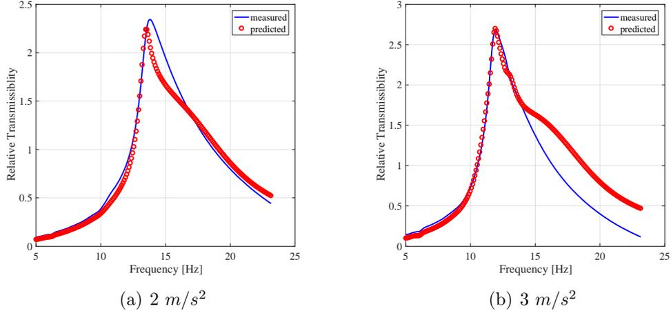
Figure 13. Comparison between measured and identified responses
