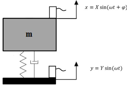
Figure 1. SDOF system of a mass suspended on a nonlinear mount with complex stiffness and under base excitation
