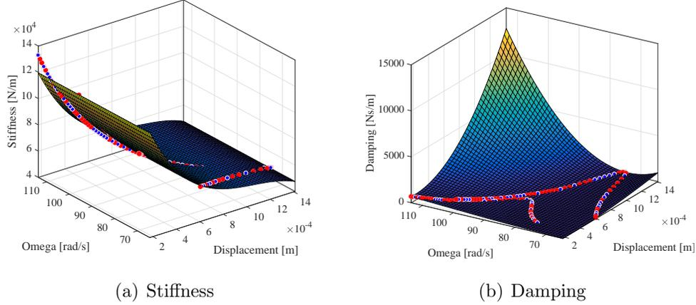
Figure 12. a) Stiffness and b) damping map of metal mesh damper including calculated points from measured data
