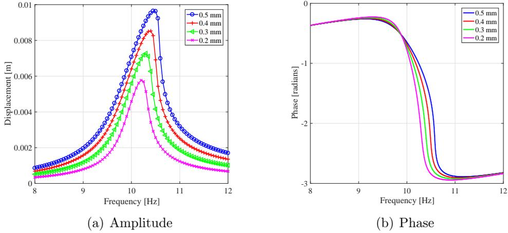
Figure 4. The response of the combined cubic stiffness and quadratic damping system for different levels of excitation
