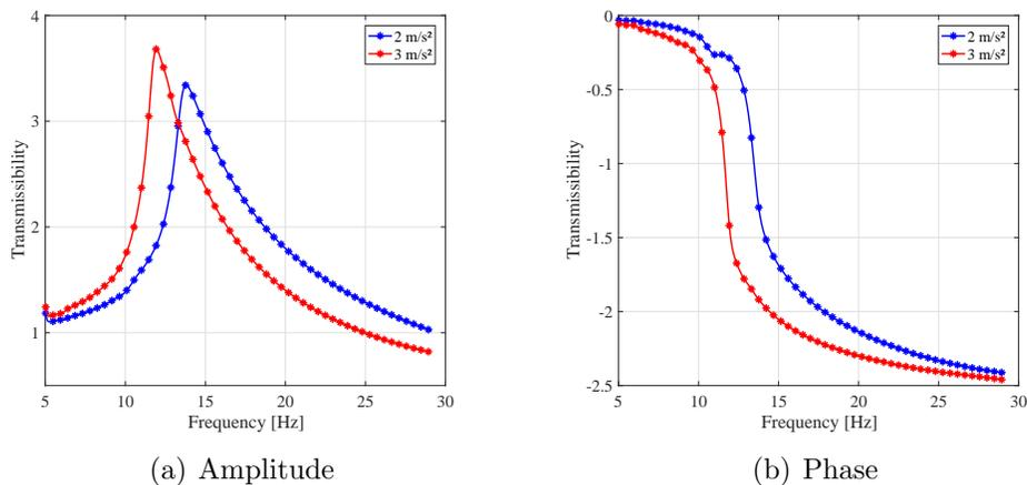
Figure 9. Acceleration responses to stepped-sine excitation of different amplitudes (a) amplitude responses and (b) phase responses
