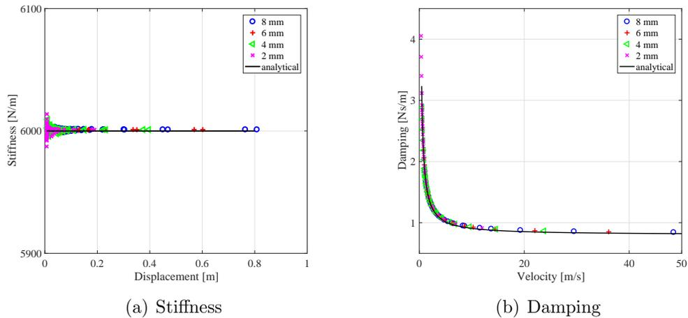
Figure 6. Comparison between the estimated stiffness and damping functions and the analytical equivalent functions: System with Coulomb damping
