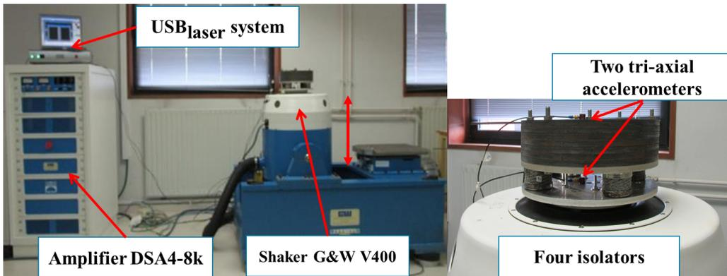
Figure 8. Experimental set-up
