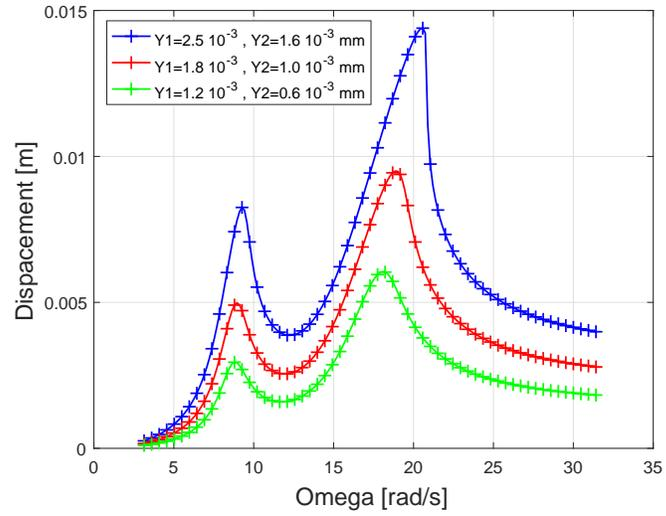
Figure 14. Response of SDOF excited by two harmonic excitations
