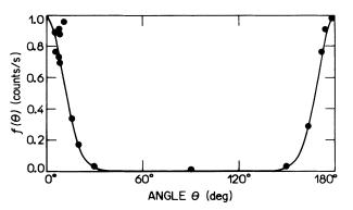
FIG. 2. Excited-state transmission between the mirrors as a function of the angle  $\theta$  between the magnetic field and the normal to the plates. Solid line corresponds to (3.7) normalized to the maximum counting rate (30 counts per second [36]).
