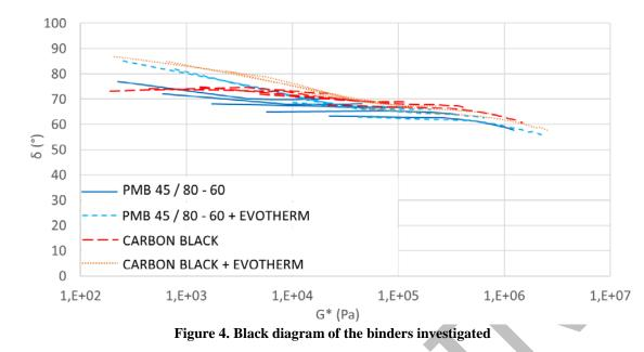
Based on the results, the performance of the experimental binder with carbon black is very similar to the commercial polymer-modified binder. In fact, the impact of Evotherm is quite similar in both binders, increasing the phase angle approximately in the same proportion for the lower stiffness; this is at high temperatures and low frequencies, as it can also be seen in Figure 4. In the case of higher stiffness, this increase is less significant.
