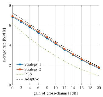
Fig. 5. Average achievable rate for the different techniques as a function of the gain of the cross-channel,  $\mathbf{H}_{ps}$ . The number of antennas is N = M = 2.
