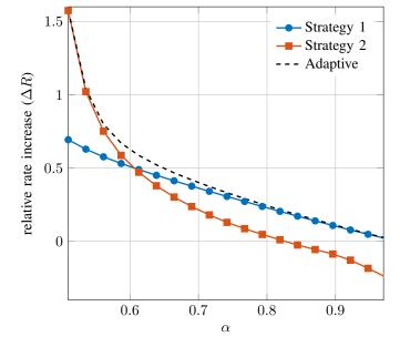
Fig. 3. Relative increase in achievable rate for the different IGS strategies as a function of  $\alpha$ . The power budget constraint is not active and the number of antennas is N = M = 2.
