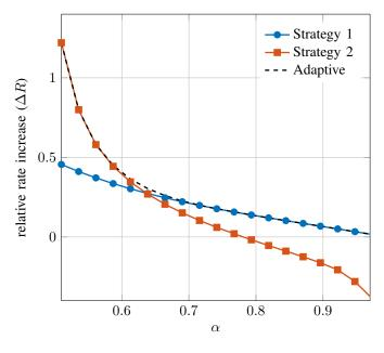
Fig. 4. Relative increase in achievable rate for the different IGS strategies as a function of  $\alpha$ . The power budget constraint is not active and the number of antennas for both users is N = M = 4.
