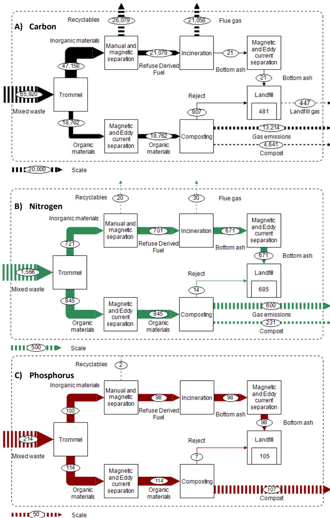
**Figure 3.1.** Flows of C (Figure 3.1.A), N (Figure 3.1.B) and P (Figure 3.1.C) in the Cantabrian mechanical biological treatment plant ( $\text{ton}\cdot\text{year}^{-1}$ ). Estimation performed with the data from the Cantabrian waste management plan<sup>2</sup> and the elemental composition of the waste components provided by the EASETECH (Environmental Assessment System for Environmental Technologies) 2.3.6 software.<sup>3</sup>
