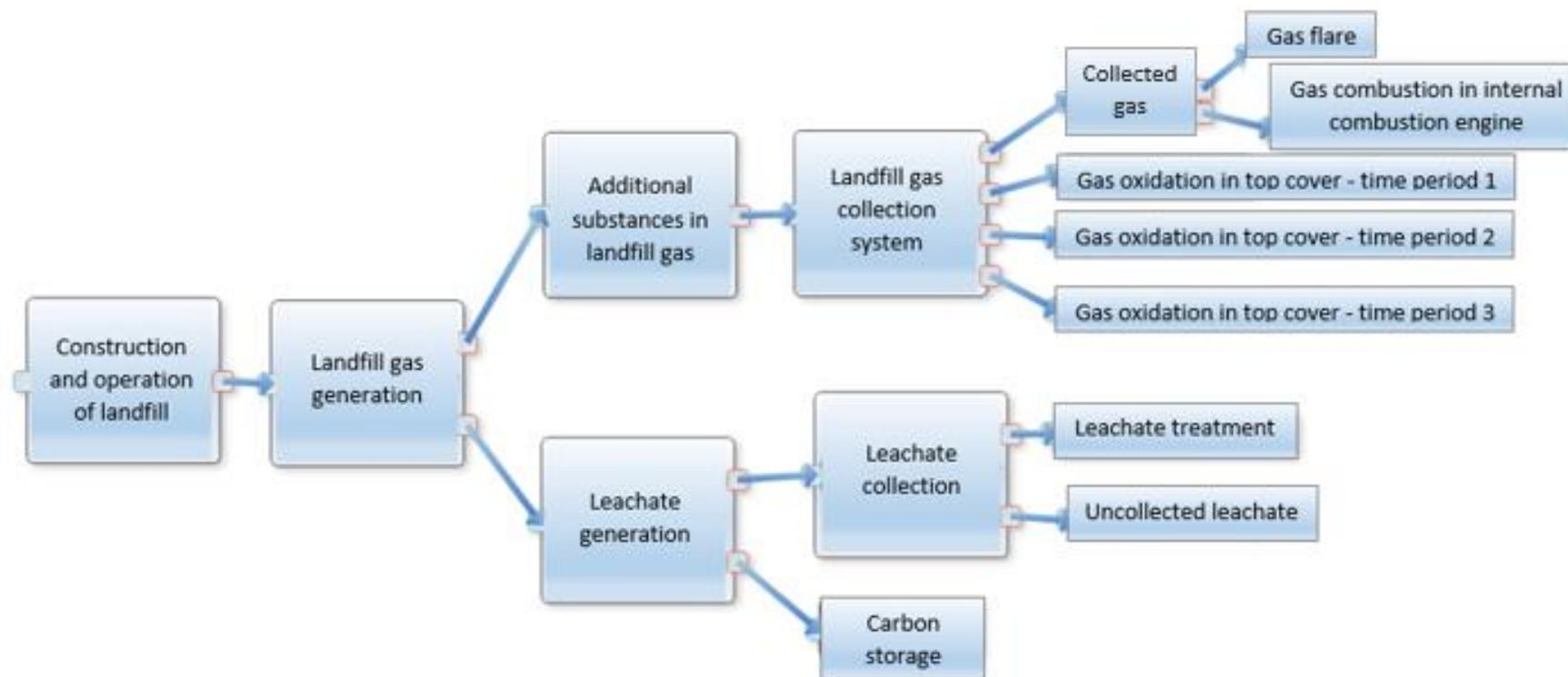
Figure S1. Sub-models of the landfill unit process
