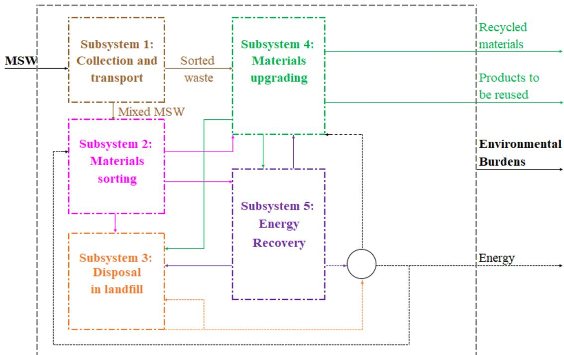
Figure 3.1.2. Configuration and boundaries of a linear IWMS
