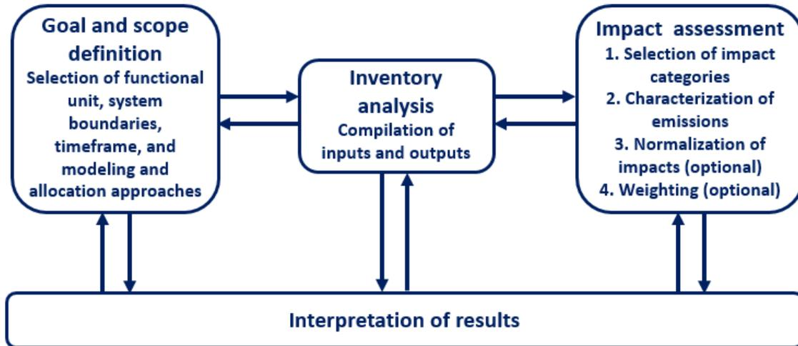
**Figure 2.4.** Overview of the LCA phases (adapted from ISO 14040<sup>8</sup>)
