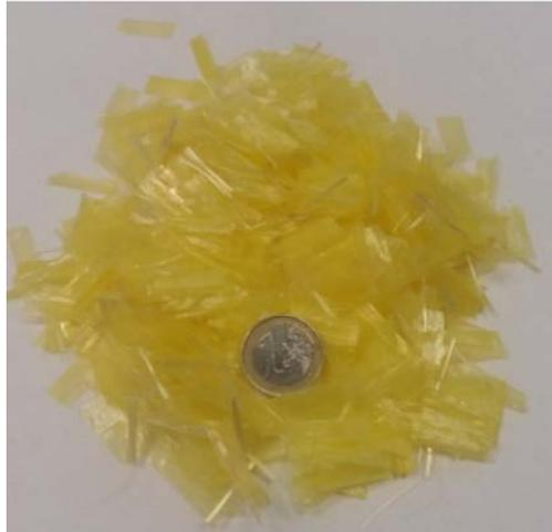
Figure 2. Blend of polyolefin and aramid (POA) fibers.
