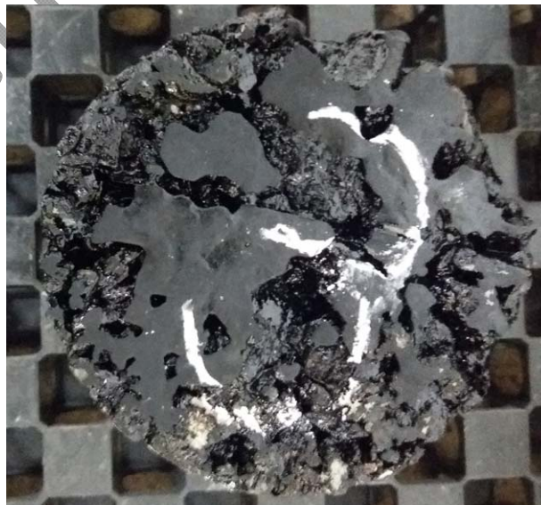
80 81 Figure 3. Bottom of a Marshall sample presenting a drainage problem after heating by induction
