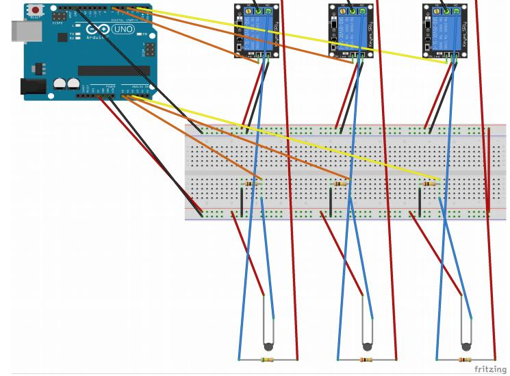
Electrical scheme of the system that allows to maintain the agarose above its melting point.
