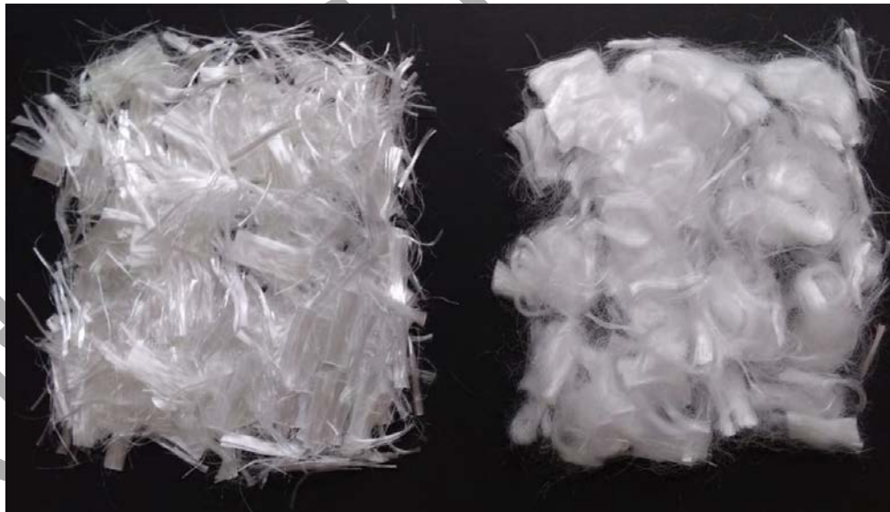
Figure 3. Fibers used in the study: Nylon (left) and PP (right).
