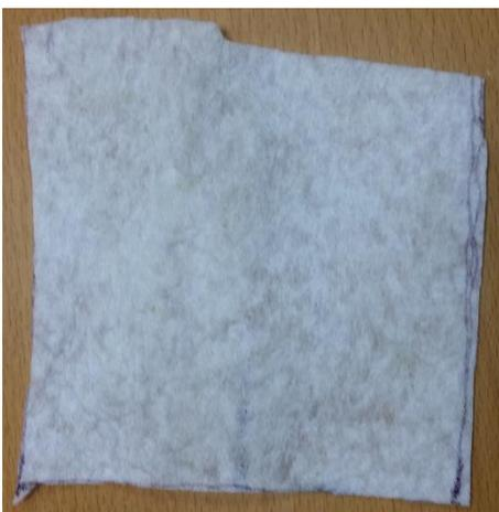
Figura 4-16. Geotextil no tejido blanco  $100 \text{ g/m}^2$  (EXP19008-1)
