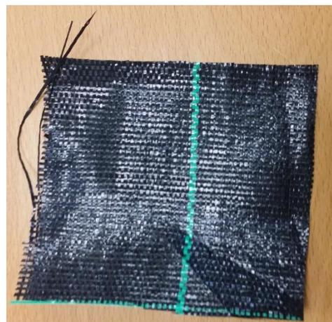
Figura 4-17. Geotextil tejido negro-tela cobertura solo PP  $100\text{g/m}^2$  (EXP19008-2)
