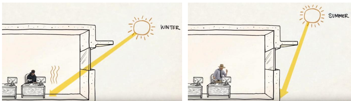
Fig. 24 How to take advantage of the sun in winter time and avoid it in summer by solar shading. (Source: Autodesk)
