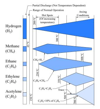
Figure 3. Gas generation based on temperature (Not to scale) [45].
