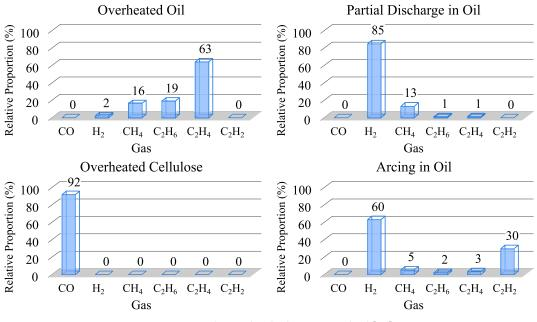
Figure 4. Fault type by the key gas method [34].
