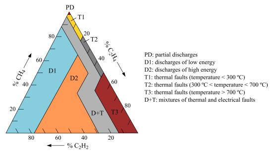
Figure 5. Duval Triangle and list of faults detectable by DGA [37].
