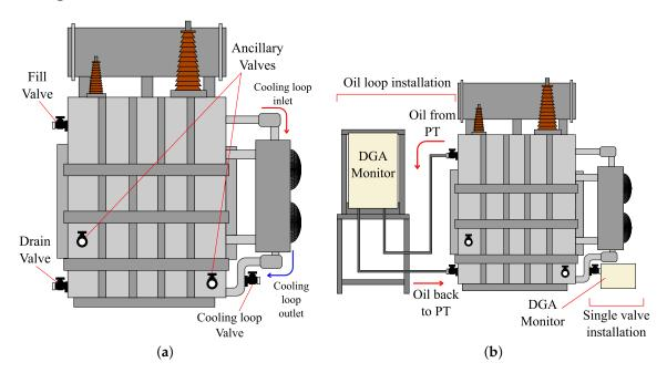
Figure 6. (a) Possible valve locations in a power transformer; and (b) installation schematic (Not to scale).
