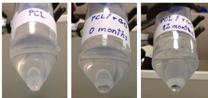
**Figure 3.6.** rGO content of the PCL/rGO membranes at 0 and 12 months of degradation.
