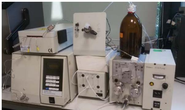
**Figure 3.2.** Gel permeation chromatography (GPC) system.
