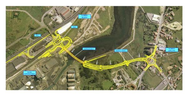
Works are located in a marisma area, so ground isn't resistent and can not be used to form the embankments. To minimice costs, two landfills are set, one on each edge of the estuary, really close to the works.
