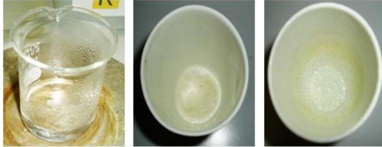
Figure 3.3: Sol, gel, and powder steps during the GGG and YAG nanoparticles synthesis by Pechini's method at the Biotechnology Department, University of Verona.
