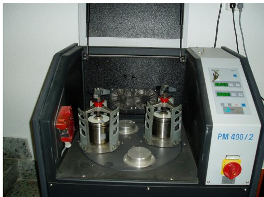
Figure 3.1: Planetary ball mill used for the synthesis of  $\text{Y}_2\text{O}_3$ ,  $\text{NaYF}_4$  and  $\text{CdS}$  nanoparticles at the Solid State Physics laboratory, University of Cantabria.
