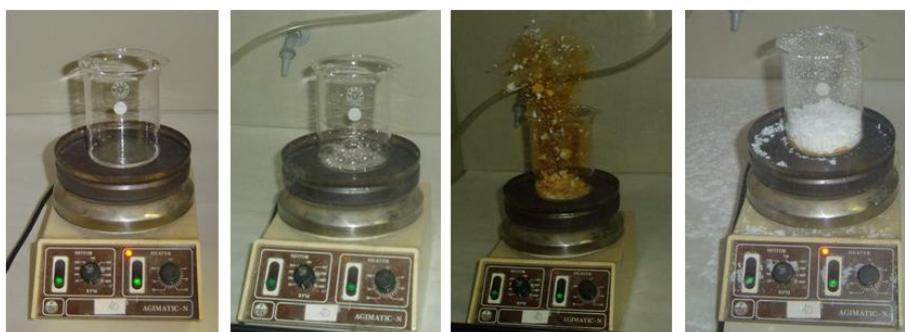
Figure 3.2: Different sequences during the combustion synthesis of RE-doped  $Y_2O_3$  nanoparticles at the Inorganic Chemistry laboratory, University of Cantabria.
