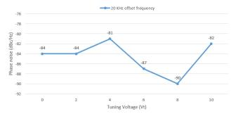
Fig 11 Measured phase noise at 20 KHz frequency offset from the carrier versus tuning voltage
