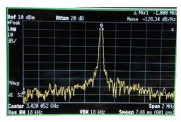
Fig. 9 Output spectrum of 2 MHz span at upper band
