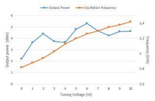
Fig 7. Measured output power and oscillation frequencies of the developed wideband VCO
