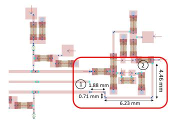
Fig. 4. Length of the transmission line to achieve the "Barkhausen oscillation criteria"
