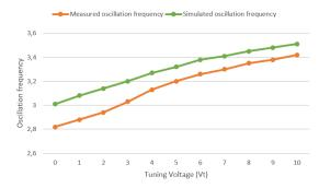
Fig. 8. Comparison between the measured oscillation frequency and simulated oscillation frequency.
