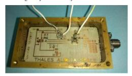
Fig. 6. Circuit photograph of the voltage controlled oscillator designed
