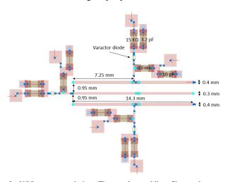
Fig. 2. VCO resonator design. Three pole combline filter and varactor polarization network
