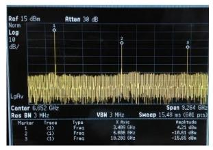
Fig. 12. Measured wideband output spectrum of the developed hybrid VCO
