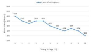
Fig. 10. Measured phase noise at 1 MHz frequency offset from the carrier versus tuning voltage
