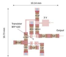
Fig. 1. Hybrid VCO core design.
