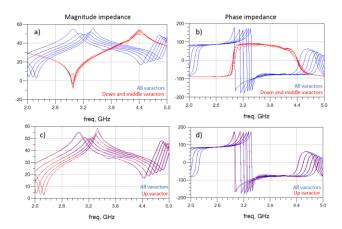
Fig. 3.(a) Magnitude comparison using all varactor diodes with down and middle varactor diodes, (b) phase comparison using all varactor diodes with down and middle varactor diodes, (c) magnitude comparison using all varactor diodes with up varactor diode, and (d) phase comparison using all varactor diodes with up varactor diode.
