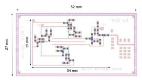
Fig. 5. Hybrid VCO Physical dimensions
