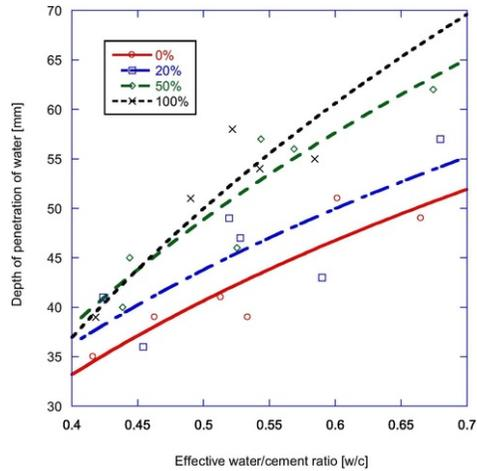
Fig. 7 Water deep penetration of recycled concretes with 28 days cured into marine environment.
