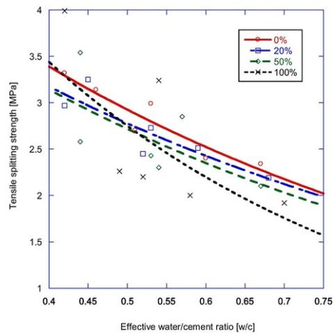
Fig. 3 Tensile splitting strength of recycled concretes with 28 days cured into marine environment.
