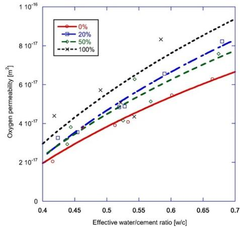
**Fig. 8** Oxygen permeability of recycled concretes with 28 days cured into marine environment.
