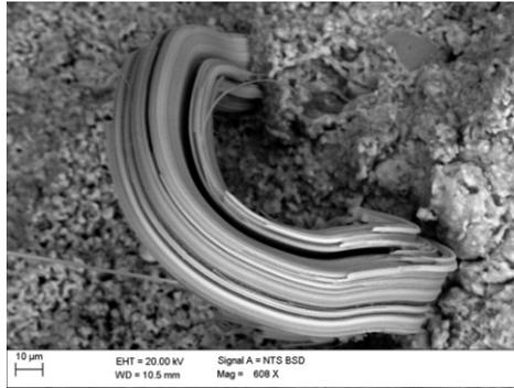
**Fig. 13** Detail of a tin whisker found into a tested sample after salt fog exposure.
