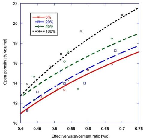
Fig. 6 Open porosity of recycled concretes with 28 days cured into marine environment.
