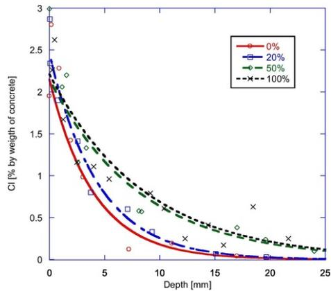
**Fig. 9** Cl weight detected in the cement paste vs. the depth from the exposed outermost surface.
