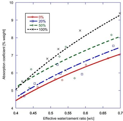
Fig. 5 Absorption coefficient of recycled concretes with 28 days cured into marine environment.
