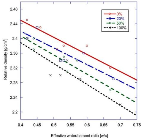
Fig. 4 Relative density of recycled concretes with 28 days cured into marine environment.
