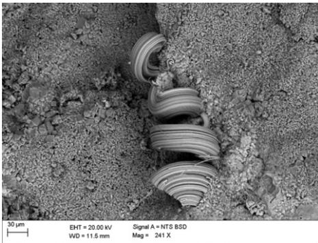
**Fig. 12** Micrograph of tin whiskers found into a tested sample after salt fog exposure.
