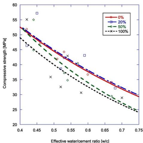
**Fig. 2** Compressive strength of recycled concretes with 28 days cured into marine environment.
