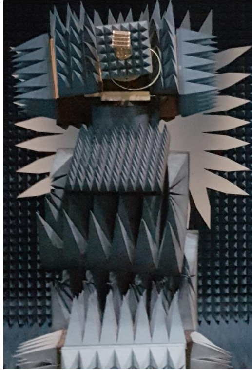
Figure 4.18 Pattern measurement of the 4x4 antenna array in anechoic chamber.
