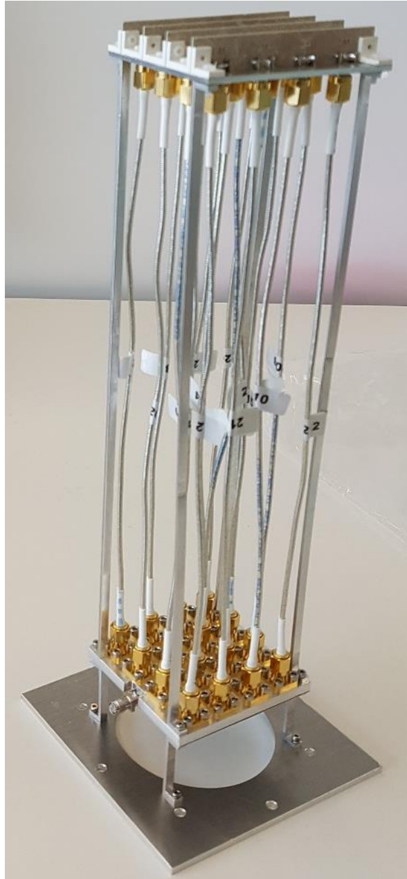
Figure 4.17 Fabricated antenna array with phasing network.
