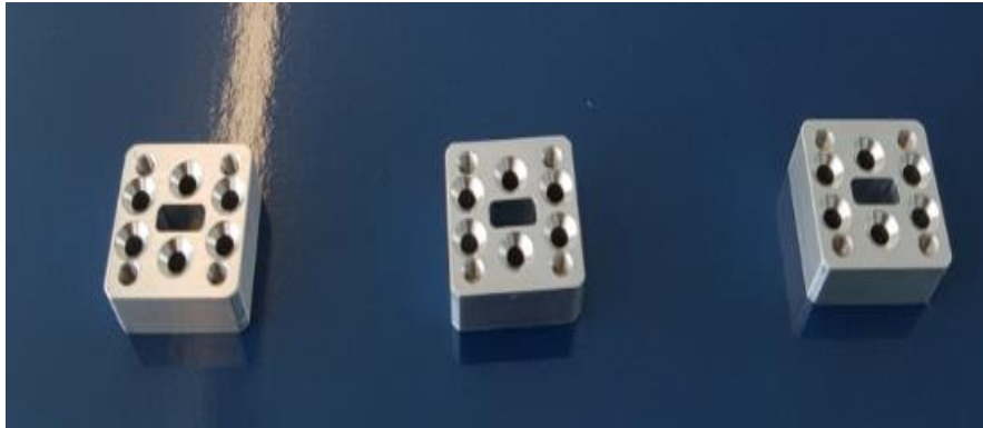
Figure 6.14 WR28 to custom horn aperture transitions for the three ports
