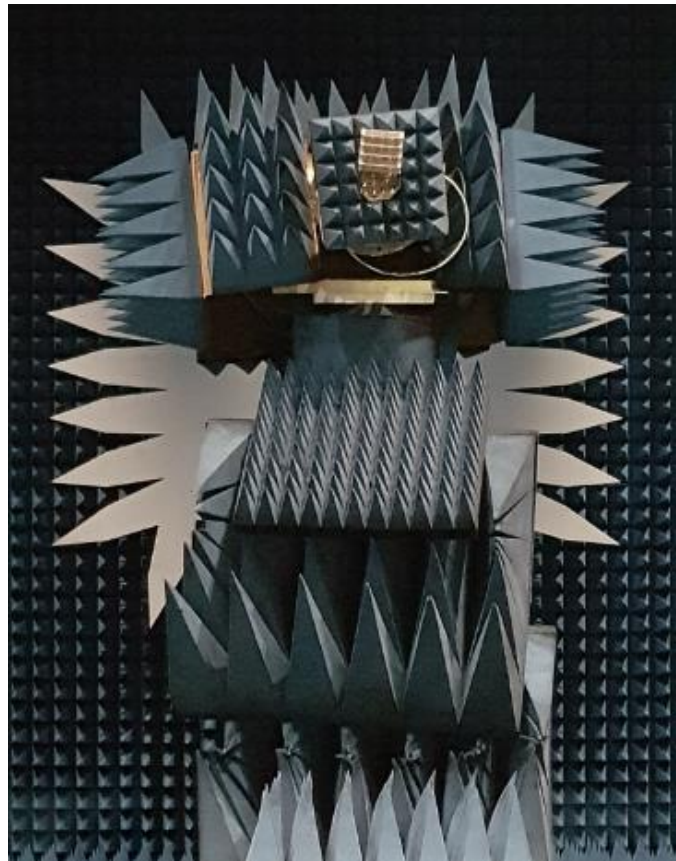
Figure 5.22 Antenna measurement setup in anechoic chamber
