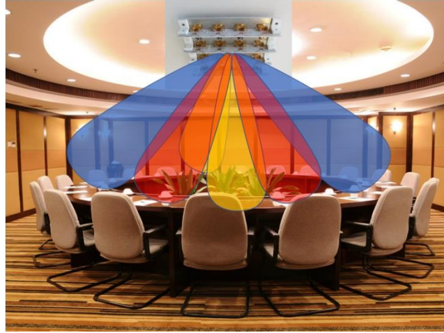
Figure 5.2 Indoor twin beam antenna for non-boresight multi-user azimuthal coverage
