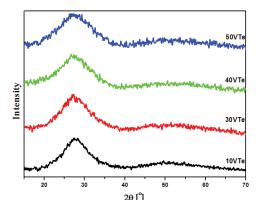
FIGURE 1. XRD patterns of V<sub>2</sub>O<sub>5</sub>-TeO<sub>2</sub> glasses.
