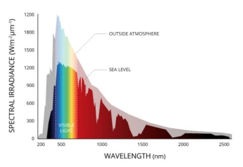
Figure 1 – Spectral distribution of solar irradiance, outside the atmosphere and at sea level. The total area equals  $G_{0\lambda}$  (data source: Gueymard 2004).
