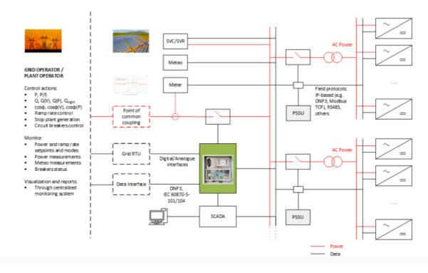
Figure 21 - Inaccess power plant controller. Source: Inaccess PPC Operating Manual v2.7
