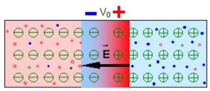
Figure 8 – Movement of electrons trough a boron-phosphoron cell
