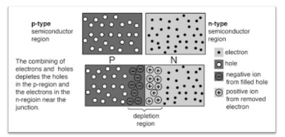
Figure 9 - P-N type cells
