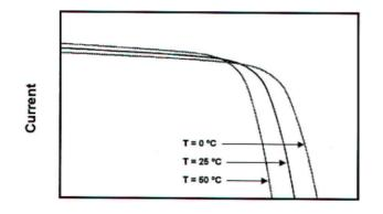
As temperature increases, the band gap energy decreases, because the crystal lattice expands, and the interatomic bonds are weakened. Therefore, less energy is needed to free an electron and move it to the conduction band."3
