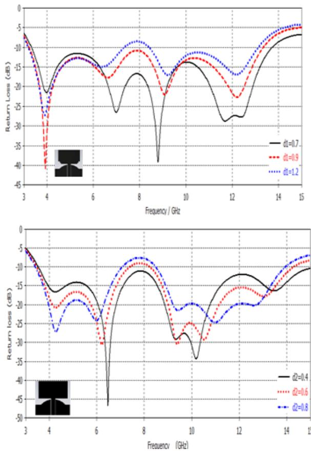
Fig.3. Effects of parameters  $d_1$  and  $d_2$  on the reflection coefficient of antennas
