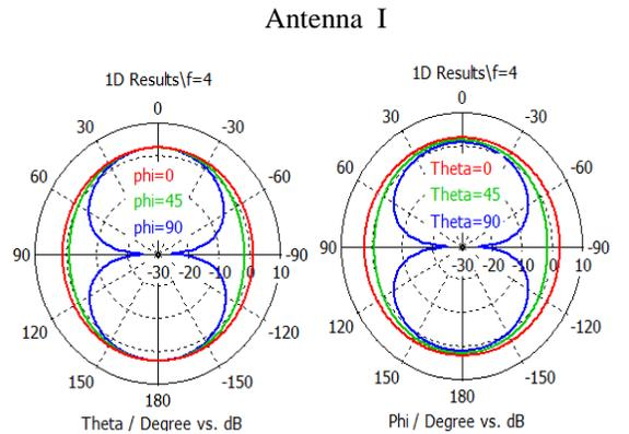
Fig.8. Simulated Gain of the proposed antennas.
