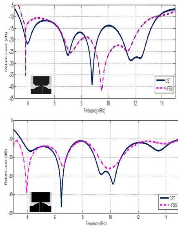
Fig.6. Comparison between reflection coefficients obtained by HFSS and CST-MW for the proposed antennas.
