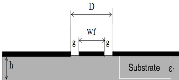
Fig.1. The definition of the main parameters for the analytic model
