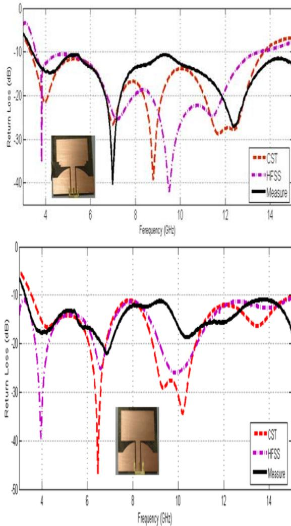
Fig.11. Simulated and measured reflection coefficients vs frequency of the proposed antennas
