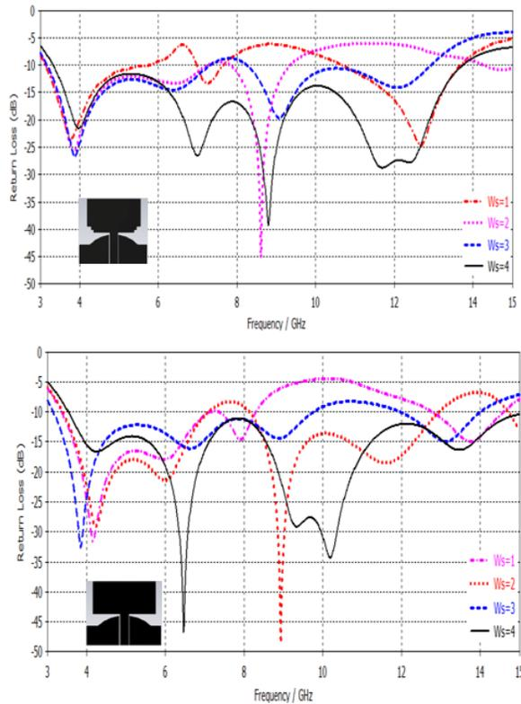
Fig.5. Effects of parameter  $W_s$  on the reflection coefficient of antennas
