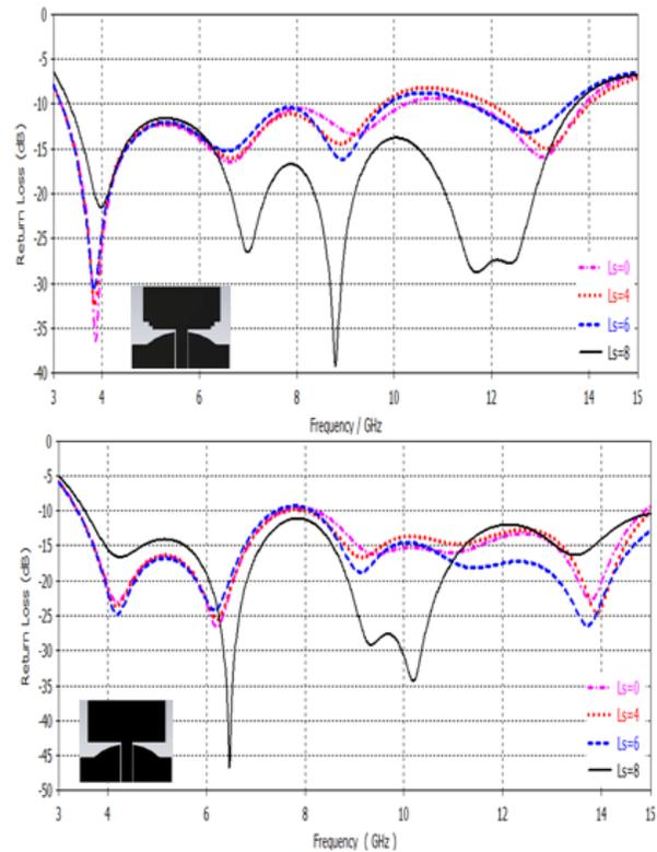
Fig.4. Effects of parameter  $L_s$  on the reflection coefficient of antennas
