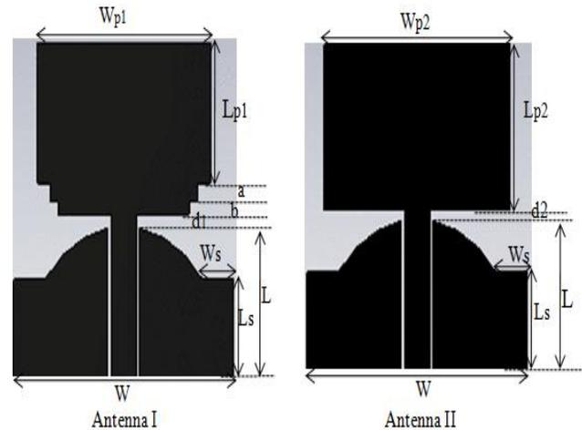
Fig.2. Geometry of CPW-fed the proposed antennas
