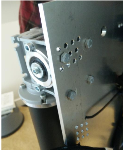
Figure 35: Picture of other perspective of the elevation motor mounted on the structure.
