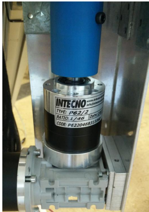
Figure 32: Picture of one perspective of the azimuth motor mounted on the structure.
