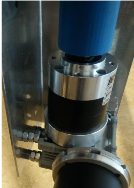
Figure 33: Picture of other perspective of the azimuth motor mounted on the structure.
