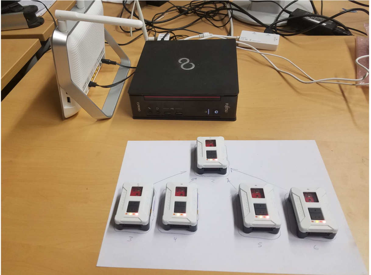
Figure 8.4.: Photo of the test bed during the Single Cluster Head Topology, Together Test. In the photo the WLAN access point (WiFi Router, Left), the sink (Computer, Center) and the five wireless sensors (XDKs, Front) can be clearly seen.
